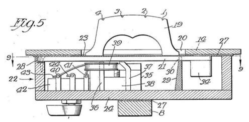
A further increase in the directness of the coupling of a stringed instrument to a magnetic coil was introduced around 1930 by Miessner [5] and others, in which the vibrations of strings made of permeable magnetic material (such as steel) cause variations in the magnetic flux through a pickup coil wrapped around a permanent magnet, as sketched in the figure on the next page.
