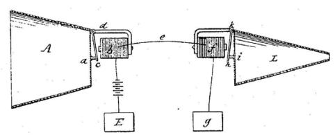
A more direct coupling between musical instruments and magnetic coils was introduced by Lloyd Loar, an instrument maker for Gibson, in the 1920's [3, 4]. In Loar's electrical stringed instruments the vibrations of a sound board actuated the pickup coil (which term Loar used), as sketched in the figure below.
