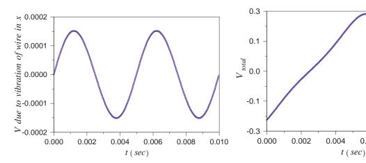
A Fourier analysis [12] of these voltage waveforms is shown in the figures below. The left figure is the voltage due to the x vibration of the string, and has significant frequency components only at the second and fourth harmonics. The right figure is the total induced voltage (almost entirely due to the y vibration of the string), which contains frequency components at all harmonics of the fundamental, with exponentially decreasing strength as a function of the harmonic number.
